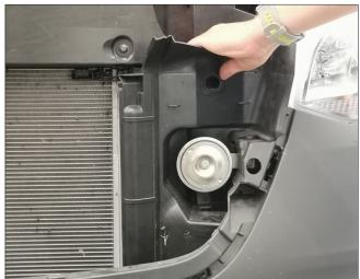
Remove cover's on both sides that are located behind the grille.
