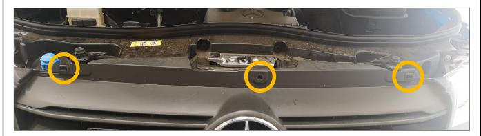
Remove the 3x Screws holding in the grille, and remove the front grille.
