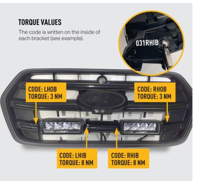
INSTALLATION PROCESS - Install should be completed with the grille left on the vehicle.
