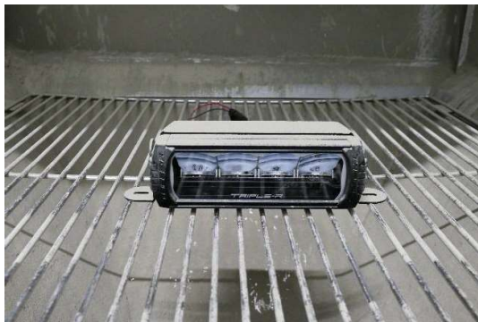
Sample after dust test
