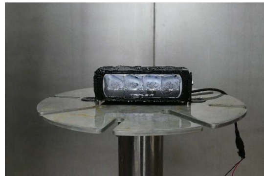
Sample after moisture test
