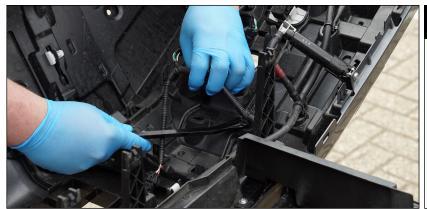
Move the wiring harness out the way of cutting area (where you have masked on the front).
