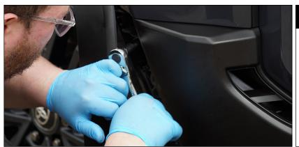
Unclip arch extensions and remove the hidden fixings, 2x 10mm bolts, 2x push rivets per side.
