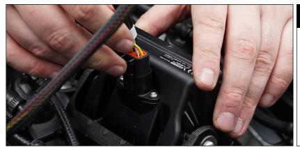
Connect the Triple-R harness to the lamps.
