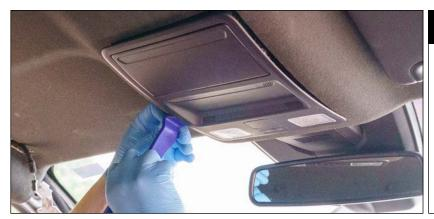
Using a trim tool, release the central roof console.
