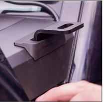
Remove 3M VHB backing from the additional cover and stick on over bracket to cover the cut.
