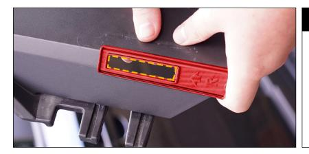
Use the cutting guides to mark out the entry holes through the top covers, and cut out with Stanley knife or similar.
