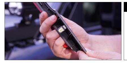
Remove small yellow clip from inner wing if left on the vehicle.
